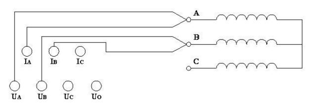
After the winding under test is wired and the suitable measuring current is selected, press the "Measure" key-press to allow the tester to enter into its measuring state and to start to supply power to the winding, and then it enters into the interface as follows:
