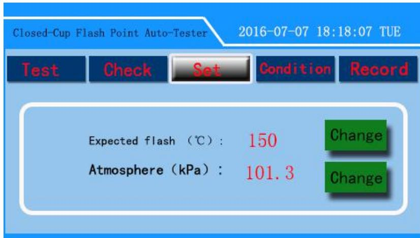
The interface can set expected flash point and the atmospheric pressure value: click "Expected flash" or "Atmosphere(kPa)" corresponding "change" into the expected flash point or pressure setting interface:
