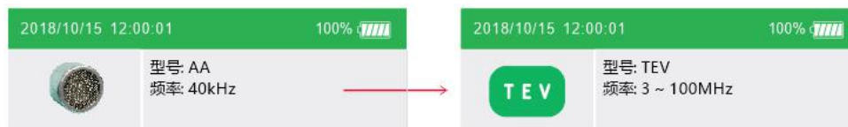
Switch from built-in sensor to built-in TEV sensor
