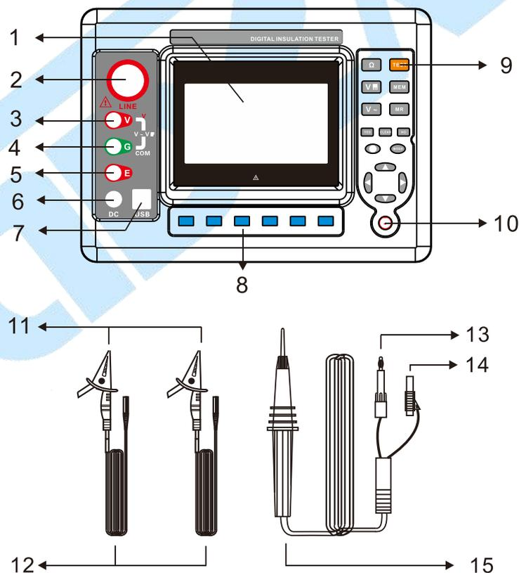
1. LCD display screen      2. LINE interface      3. V interface
