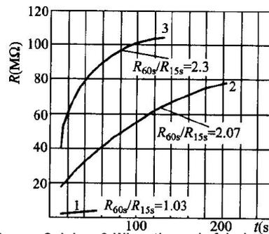
1-Befor drying,15 degree Celsius; 2-When the end of drying, 73.5 degree Celsius
