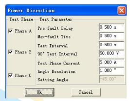
value of the largest sensitive angle has been used in the software. Suppose the largest sensitive angle of protection is  $-45^{\circ}$ , no matter users input  $-45^{\circ}$  or  $+45^{\circ}$ , there is not any influence on normally test. The right diagram shows the dialog box for setting parameters.
