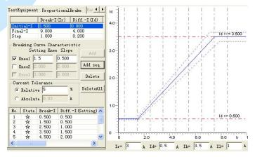
it is not effective in the mode of bidirectional approaching. Set step size of difference current according to the precision of protection. If high precision is required, the step size should be set smaller.
