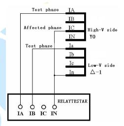
△ side has phase adjustment, connecting in single phase short circuit mode.
