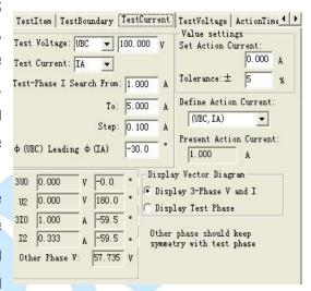
current, the angle is positive. So please pay attention to the positive angle and negative angle when setting angles. Normally, when the setting angle is equal to or near sensitive angle, the protection acts the most sensitively, and the action current tested also is the mose exact. When the setting angle is deflected too much, the action current tested may be larger or even relay may not act.
