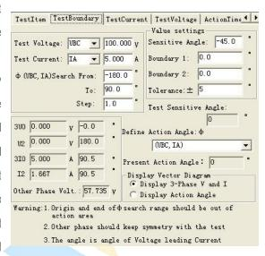
the selected voltage and current can be set, but the voltages of unselected phases are equal to rated voltage and symmetrical, and the currents of those phases are 0.
