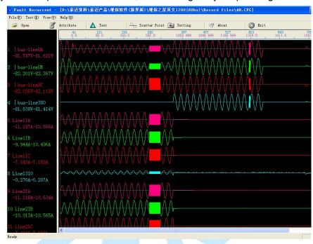
After ending the test, computer will file the testing result in the subentry of 'test report\fault reappearance' in text format, and it can be displayed or printed by pressing the 'print' key. You can also copy it to be compiled or amended by compiling tools like WORD.
