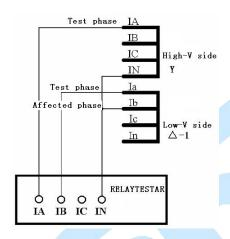
Y side has phase adjustment, not zero sequence. connecting in single phase short circuit mode.
