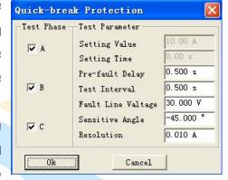
mouse. After that, set other testing parameter in a dialog box ejected. We hereby take 'quick break protection' as the example for detail explanation. See the right diagram:
