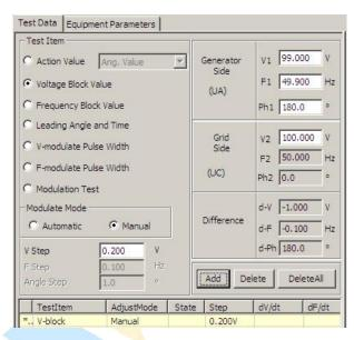
When any one of the above-mentioned parameters needs to be tested, you should always make other two parameters satisfy synchronization condition in advance. Through changing value of parameters needs to be tested to make the synchronous device to act finally after satisfying fully synchronization requirements.
