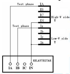
There is phase adjustment on two sides, but not zero sequence adjustment
