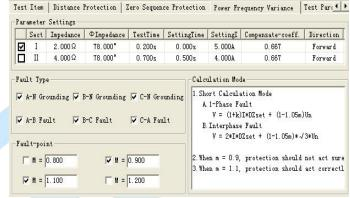
M has 0.9 and 1.1 two kinds of value in the default situation. Normally, the protection does not act reliably when M=0.9; the protection should be act reliably when M=1.1. You can measure the action time of protection when setting M=1.2
