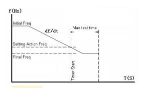
So if the setting value has deviation, it will influence the time measuring precision. For process of test, please see the right diagram.
