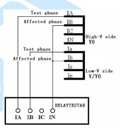
There is not phase adjustment on two sides, but zero sequence adjustment.
