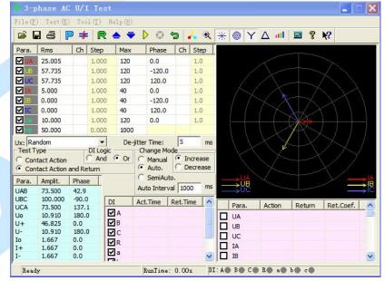
three-phase current but not actual output of single phase of tester. If changing any sequence component value on the interface (including amplitude and phase) ,software will real-time calculate corresponding three-phase voltage and current ,which will be displayed in the listing area on the lower left side of interface. The tester output voltage and current displayed on the interface rather than sequence component.
